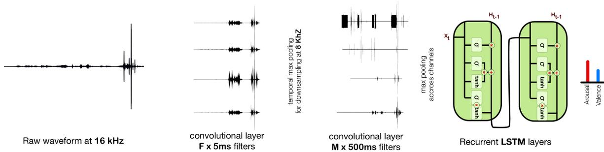
**Fig. 1.** Illustration of the proposed convolutional recurrent network topology for emotion prediction from the raw waveform signal. The convolutional layers replace the need for hand-engineering features which were used till now in the paralinguistics community.
